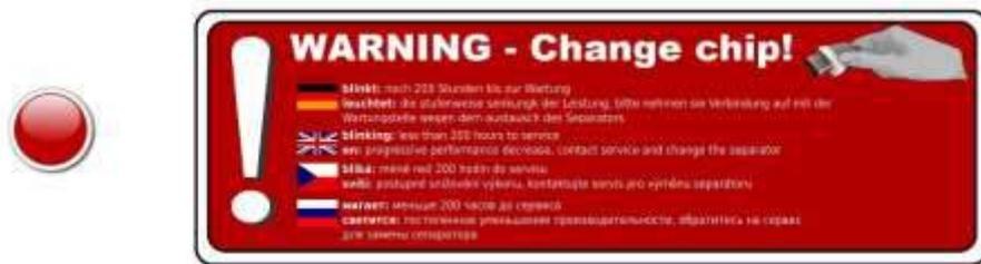
BERGCare running is indicated by a red indicator on the front panel (compressors without the control system) or directly on the control system panel of the compressor. During activation of the system (switching the machine on) the indicator blinks once to three times (according to the compressor type).
