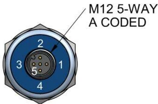
Figure 4 Sensor Connector Installation
