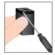
Figure 2 Connector Terminal Block Removal
